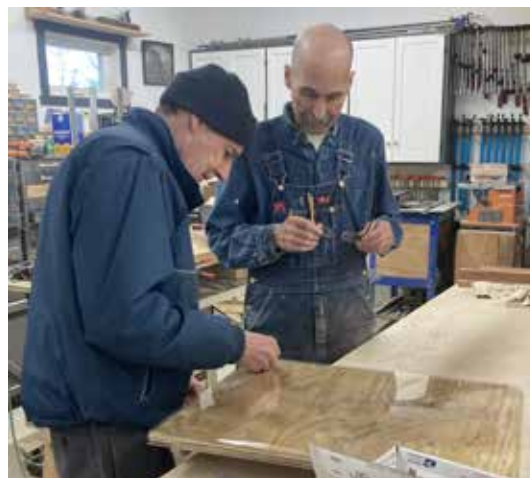
Captions left to right: Tim heating up the polycarbonate cover before bending to shape; Tim and Eric fitting the pieces together; Steve adding supports to the backer boards.
